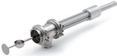
For collecting a sample in a drop tube. After retraction, the cup is tipped and the sample is emptied into a container.
