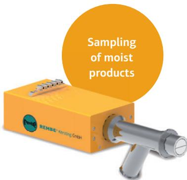
The pneumatic sampler SMARTwet has been specially developed for the “moist product” application area. It is connected directly to the process by means of a weld-on flange or clamp connection. To remove material, the sampling port moves into the process while rotating and takes up material; Subsequently the sample is pressed through a plug in the sampling tube into the outlet port of the sampler. Different collection systems can be adapted here such as bottles or a liner system.
