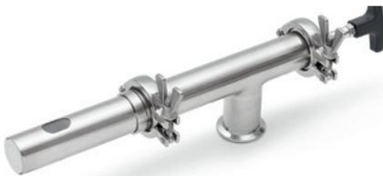
Plug samplers transport a defined amount of the product by means of a plug from the process into a downstream sample collection system. Typical use in the sampling of a material from pre-containers, e.g. at bagging plants.
